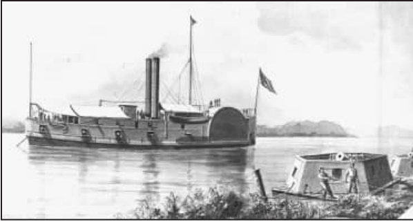
Steamboat A. O. Tyler after its conversion to the Union gunboat USS Tyler . The United States purchased the boat for $20,666 in June 1861 and remodeled her for service as a gunboat. The bulwarks around the cannon were reinforced with 5 inches of white oak against small arms fire but provided little protection against artillery. The name honors Sir Charles Tyler of the British navy, recognized for his distinguished service and bravery during the Napoleonic Wars, and subsequently bestowed with the Knight Grand Cross. (loc)
